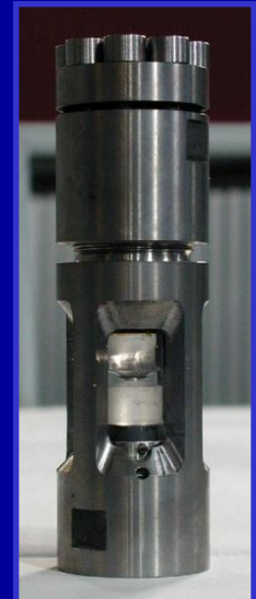
Sapphire anvil high pressure cell for DN-6
