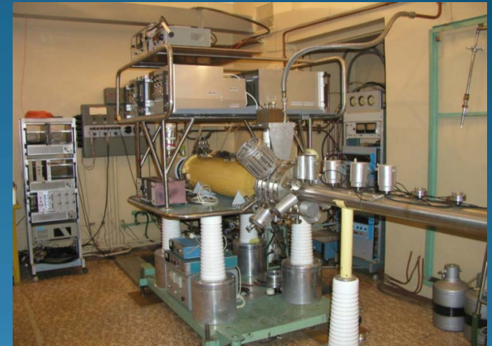
ESIS –Superconducting JINR ion source, applied for carbon ion injection
