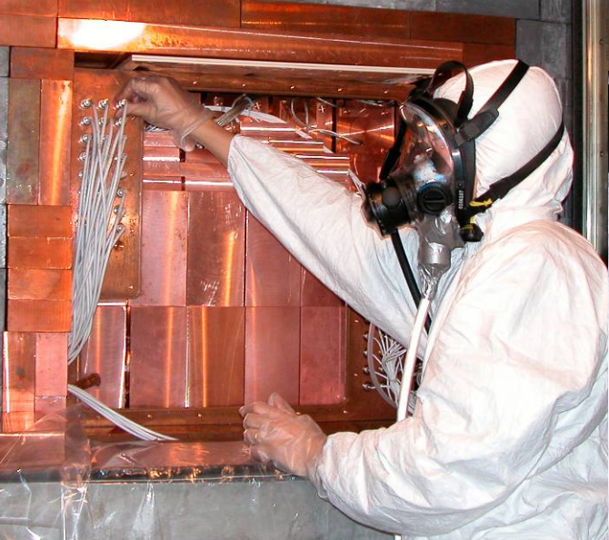
filling the inner Cu box further shield
