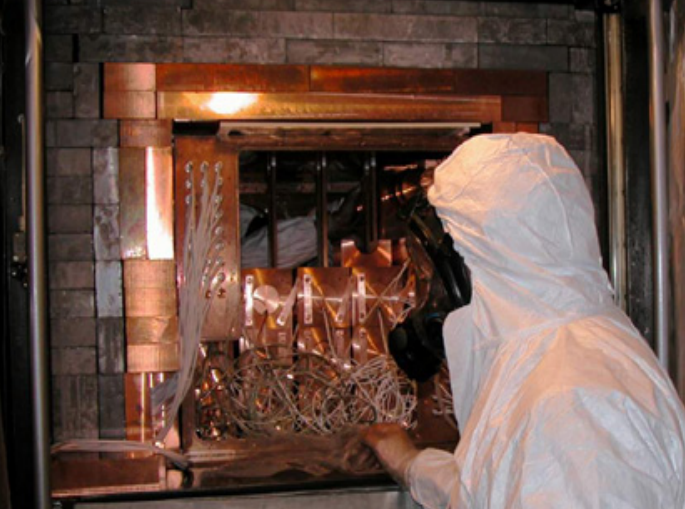
installing DAMA/LIBRA detectors
