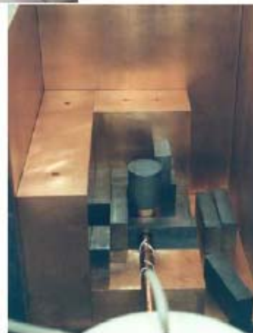
Fig. 1. The HEIDELBERG–MOSCOW \beta\beta -experiment in the Gran Sasso (top), and four of the enriched detectors during installation (bottom left). The fifth detector was installed in an extra shielding using electrolytic copper as inner shield (bottom right).
