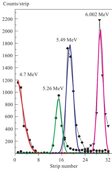
Fig. 3. The distribution of the  $^{226}\text{Ra}$   $\alpha$  source;  $\alpha$  with different energies at the focal plane of the separator. Obtained energy resolution is about 2 %, dispersion — 3.8 mm/%
