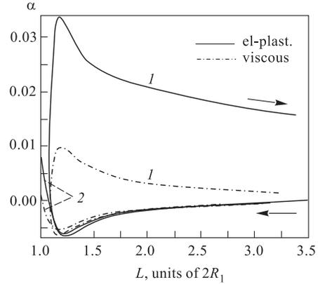
Fig. 2. Trajectories of the two-molibdenum system in  $\alpha$ - $L$  plane. Here and in the next figure the solid lines are obtained taking into account memory effects in friction forces, the broken lines correspond to the viscous approximation. Curves 1 and 2 correspond, respectively, to  $E_{\text{in}} = 4.0$  and 4.4 MeV/nucleon. Arrows beside the curves indicate the time evolution
