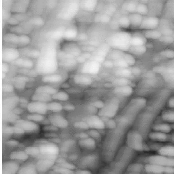
Fig. 1. The AFM image of the 700 nm (in the average) thick Nb-film. The film was prepared in Particle Physics Laboratory of JINR by electron beam evaporation. The neutron reflection roughness is 8 nm. The conditioned colors indicate the height range (0 – 40) nm (from dark-red to light-red, respectively). The AFM average roughness is 6.7 nm, which is in good agreement with neutron reflection estimation
