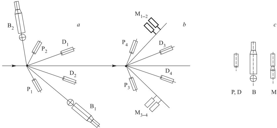
Fig. 1. The schematic view of the internal target experiment:  $P_i$  and  $D_i$  are the proton and deuteron detectors;  $B_i$  —  $\Delta E - E$  detectors;  $M_i$  — monitor counters. *a*) Horizontal plane; *b*) vertical plane; *c*) schematic view of P, D, B and M detectors
