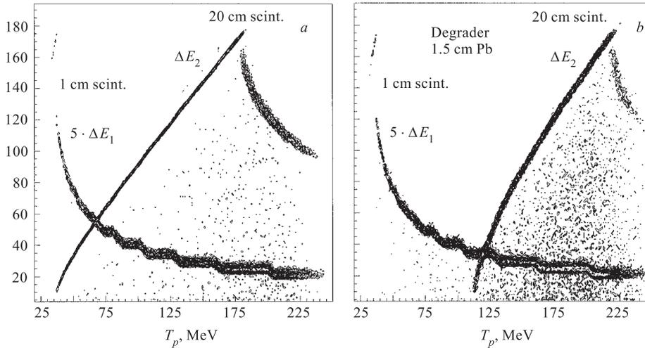
Fig. 5. Energy losses of proton in 1 and 20 cm scintillators, respectively. The lead degrader 1.5 cm thick is placed in front of the 20 cm scintillator (*b*)
