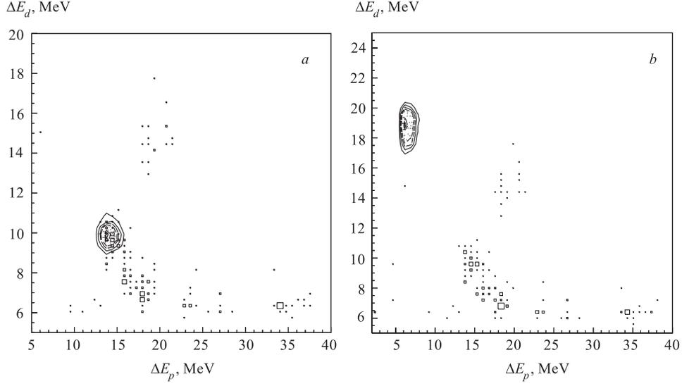
Fig. 4. Correlation of two detected-particles energy losses in 2 cm scintillators at 500 MeV and angles corresponding to the deuteron scattering angle of  $60^\circ$  (a) and  $120^\circ$  (b) in the c.m. The contour and boxes represent the events coming from  $dp$  elastic scattering and  $dp$  breakup, respectively
