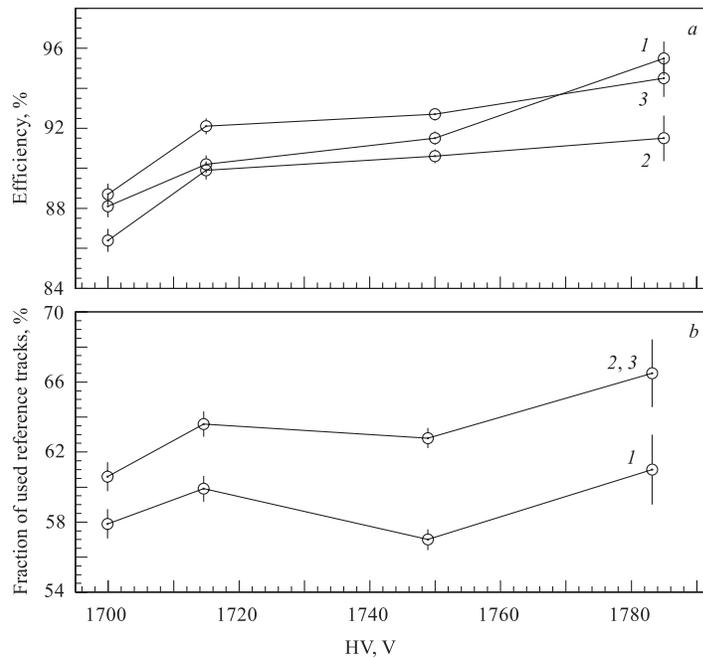
Fig. 10. High voltage scan results: *a*) dependence of the track efficiency in PC chambers on high voltage at 5-mm chambers; *b*) dependence of the fraction of used reference VDS+RICH+ECAL tracks on high voltage. The lines are labelled with the number of the method used
