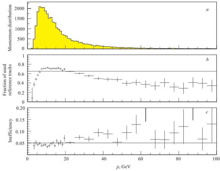
Fig. 8. Dependence of the PC chambers track-finding inefficiency on the momentum of the track
