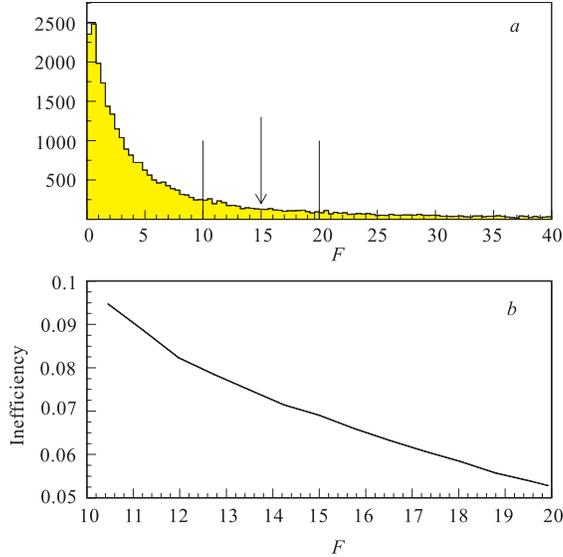
Fig. 11. Systematic uncertainties due to the choice of  $F^{\text{cut}}$ : *a*) distribution of  $F$  and the chosen cut; *b*) variation of the inefficiency according to the  $F^{\text{cut}}$  value
