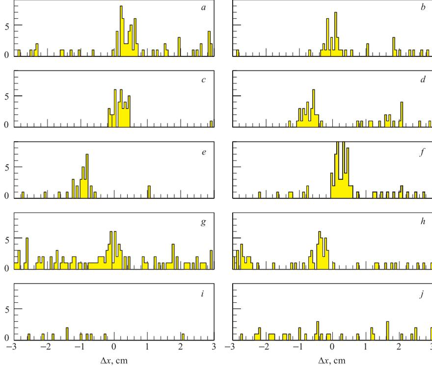
Fig. 4. Examples of histograms for the residual  $\Delta x = x^{\text{tr}} - x^{\text{hit}}$  for individual events in run 14577: *a-h*) correspond to the case of found PC segment; *i, j*) correspond to the events where no track in PC was observed
