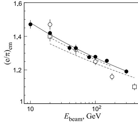
Fig. 1. The  $(e/\pi)_{em}$  ratios as a function of the beam energy for this method (black circles) and for weighting method (open circles for Ref. [12] and open squares for Ref. [13]). The lines are the result of a fit of Eq. (3) with free  $e/h$  parameter and  $k = 0.11$ : solid line is for the [23] data, dashed line is for the [12] data and dash-dotted line is for the [13] data
