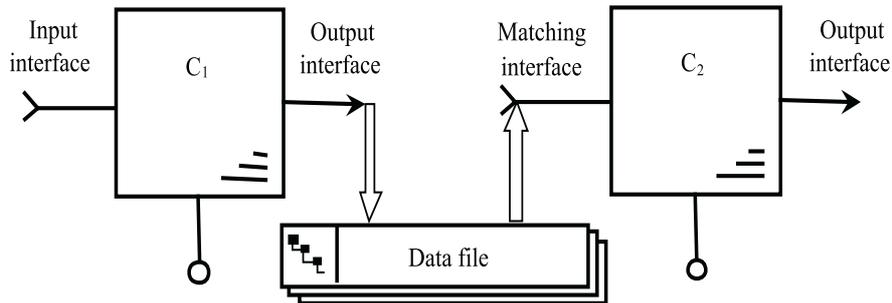
Fig. 10. Component collaboration by the data file bus
