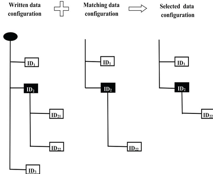
Fig. 5. Matching the tree structured data
