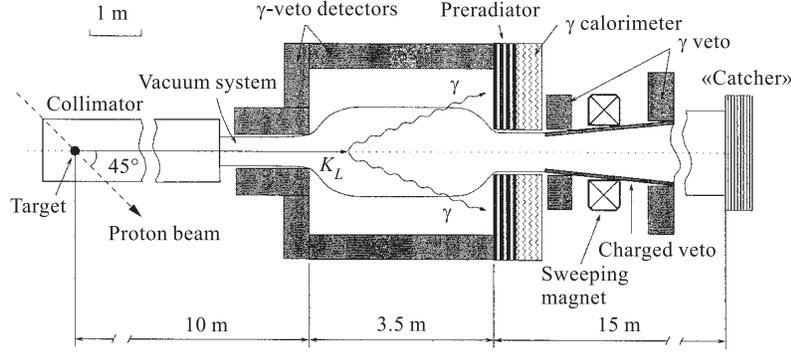
Fig. 4. Schematic view of the KOPIO experiment
