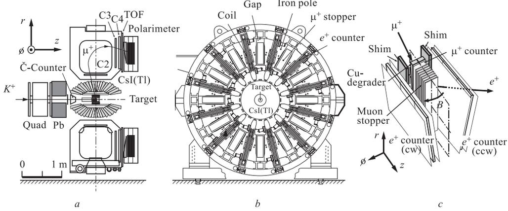
Fig. 5. The layout of the KEK E246 detector: *a*) side view, *b*) end view and *c*) one sector of the polarimeter
