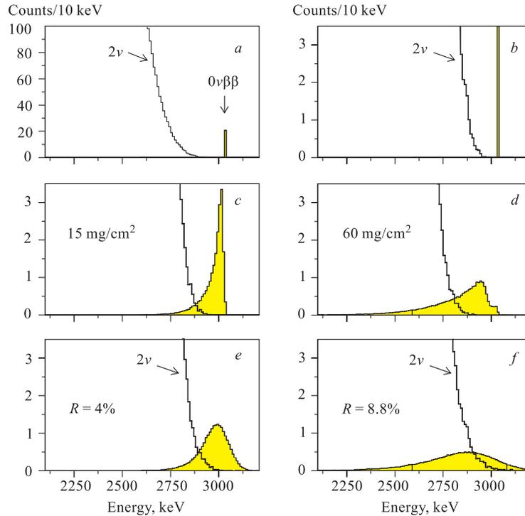
Fig. 1. Simulated spectra of the model  $2\beta$  decay experiment with 1 kg source of  $^{100}\text{Mo}$ . a) and b) «Active» source technique:  $^{100}\text{Mo}$  nuclei in a detector with 100 % efficiency, zero background, and with 10 keV energy resolution. c) and d) «Passive»  $^{100}\text{Mo}$  source in the same detector with foil thickness 15 and 60 mg/cm<sup>2</sup>. e) The same as c) but the energy resolution (FWHM) of the detector at 3 MeV is 4 %. f) The same as d) but with FWHM= 8.8 %
