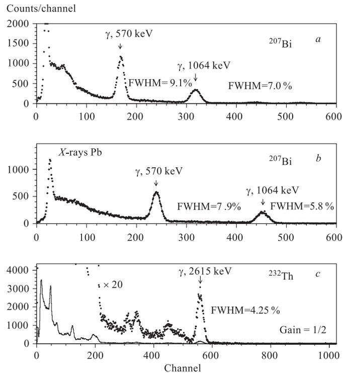
Fig. 4. The energy spectra of  $^{207}\text{Bi}$  ( $^{232}\text{Th}$ ) source measured with a  $\text{CdWO}_4$  crystal ( $\varnothing 40 \times 30$  mm) for two arrangements: *a*) standard, where the  $\text{CdWO}_4$  crystal is wrapped by teflon diffuser and directly coupled to the PMT's photocathode with optical glue; *b*) the  $\text{CdWO}_4$  crystal is located in the liquid and viewed by two distant PMTs (see text); *c*) the same as *b*) but with a  $^{232}\text{Th}$  source
