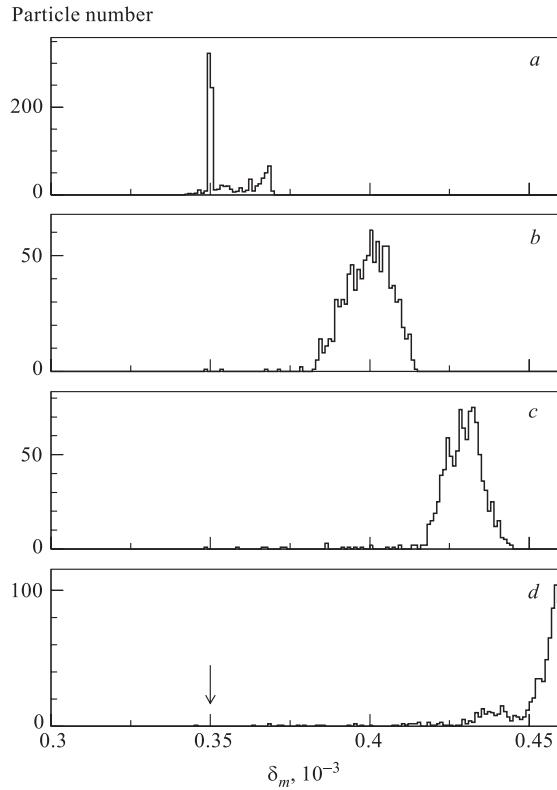
Fig. 5. The distributions of halo particles in synchrotron oscillation amplitudes  $\delta_m$  under the action of the resonance strengthening sequence at different turn numbers: *a* —  $25 \cdot 10^3$ ; *b* —  $250 \cdot 10^3$ ; *c* —  $350 \cdot 10^3$ ; *d* —  $450 \cdot 10^3$ . The pulse duration  $\Delta l_p = 2$  cm,  $N_{on} = 640$ . The arrow shows the initial amplitude of particles
