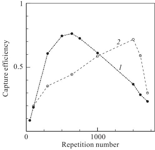
Fig. 13. The dependence of the capture efficiency of halo particles by the damping sequence on the repetition number. The initial amplitude  $\delta_{mo} = \delta_{ms}$ , where  $\delta_{ms} = 0.44 \cdot 10^{-3}$  is the start amplitude of the sequence. The pulse length  $\Delta l_p = 2$  cm,  $V_p = 0.5$  MV. The curve 1 and 2 are for decelerating and accelerating pulses correspondingly
