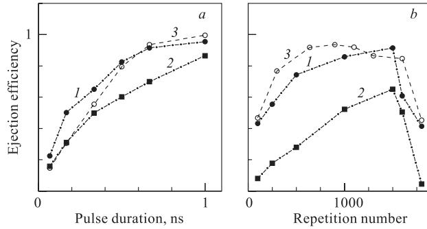
Fig. 8. The dependence of the ejection efficiency of halo particles from the bucket on the pulse duration (a) and the sequence repetition number (b). In (a) with accelerating pulses  $V_p = 1$  MV (1) and  $0.5$  MV (2),  $N_{on} = 1500$ , and with decelerating pulses  $V_p = -1$  MV,  $N_{on} = 900$  (3). In (b) with accelerating pulses  $V_p = 1$  MV,  $\Delta l_p = 20$  cm (1),  $10$  cm (2), and with decelerating pulses  $V_p = -1$  MV,  $\Delta l_p = 20$  cm (3)
