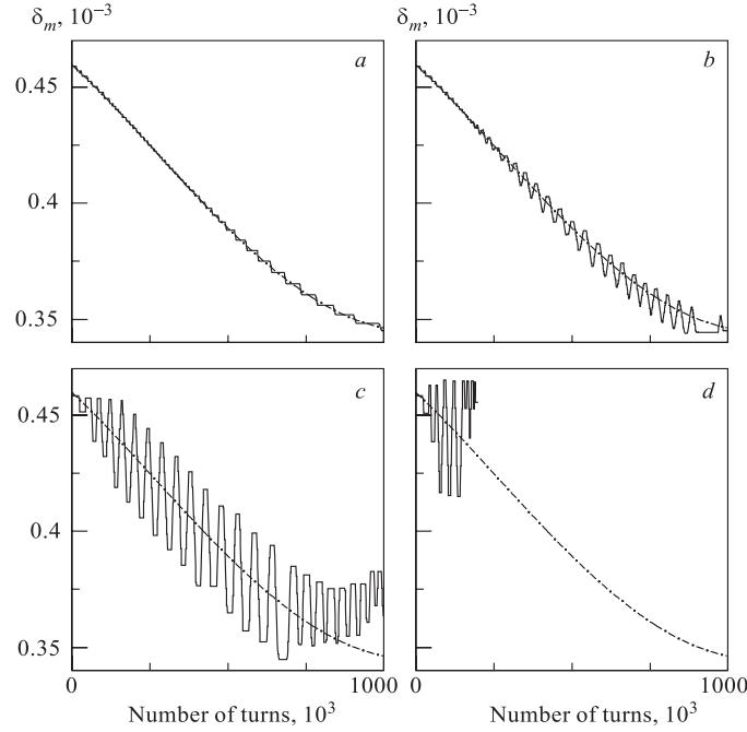
Fig. 11. The oscillation amplitude  $\delta_m$  as a function of turn number for a halo particle driven by a resonance damping sequence with different pulse length  $\Delta l_p$  and repetition number  $N_{on}$ . With short pulses  $\Delta l_p = 2 \text{ cm}$ ,  $N_{on} = 100$  (a), 1500 (b). With long pulses  $\Delta l_p = 10 \text{ cm}$  (c) and 20 cm (d),  $N_{on} = 640$ . The pulse voltage  $V_p = 0.5 \text{ MV}$
