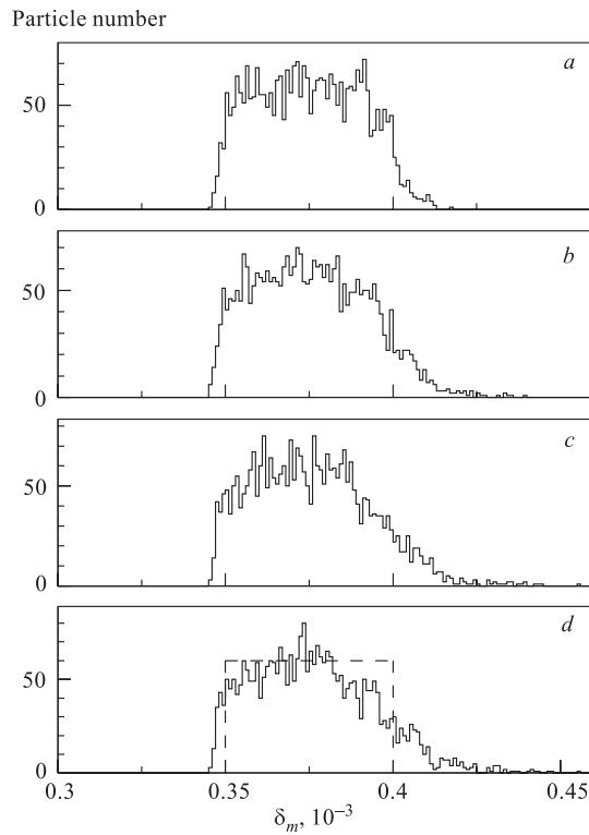
Fig. 9. The distributions of halo particles in oscillation amplitudes  $\delta_m$  under the action of the periodic sequence at different turn numbers:  $25 \cdot 10^3$  (*a*),  $225 \cdot 10^3$  (*b*),  $325 \cdot 10^3$  (*c*),  $425 \cdot 10^3$  (*d*). The pulse length  $\Delta l_p = 5$  cm, the period  $T_p/T_0 = 1620$ ,  $N_{on} = 1500$ . The initial distribution is shown by dashed line
