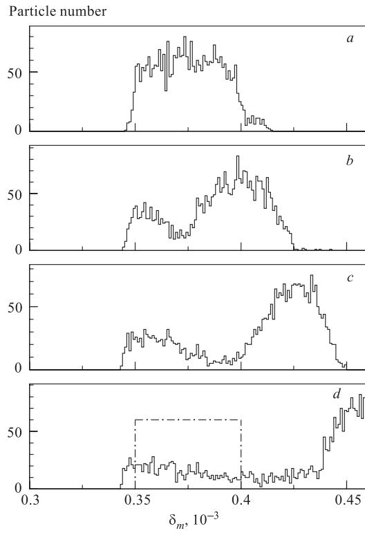
Fig. 7. The distributions of halo particles in amplitudes  $\delta_m$  under the action of the resonance strengthening sequence at different turn numbers:  $25 \cdot 10^3$  (a),  $225 \cdot 10^3$  (b),  $325 \cdot 10^3$  (c),  $425 \cdot 10^3$  (d). The initial distribution with  $\delta_{mo} = (0.35-0.40) \cdot 10^{-3}$  is uniform (dashed line). The pulse length  $\Delta l_p = 5$  cm,  $N_{on} = 1500$
