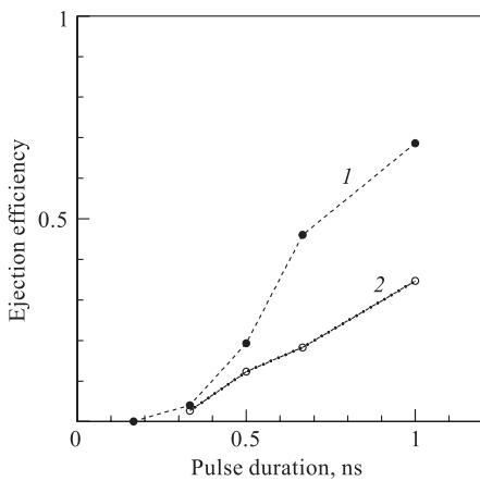
Fig. 10. The dependence of the ejection efficiency of halo particles from the bucket on the pulse duration of the periodic sequence. The sequence period  $T_p/T_0 = 3000$  (1), 1500 (2),  $N_{on} = 200$
