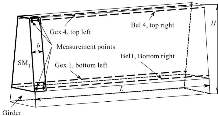
Fig. 2. Measurement lines on the MODULE surface
