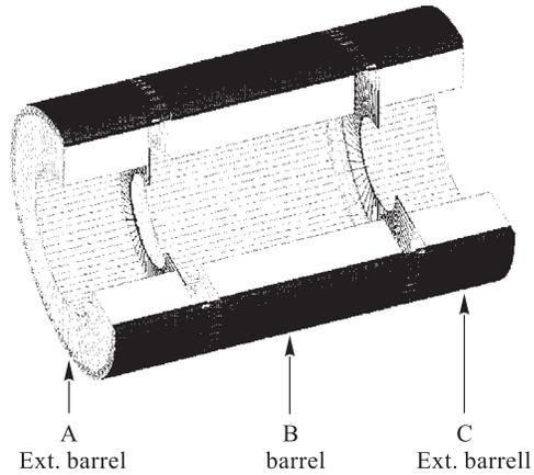
Fig. 1. The tile-calorimeter barrel and two extended barrels
