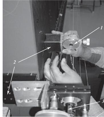
Fig. 13. Measurement system: 1 — quadrant photodiode; 2 — magnetic bases; 3 — laser
