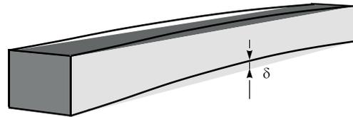
Fig. 7. Sagging («banana») of the girder
