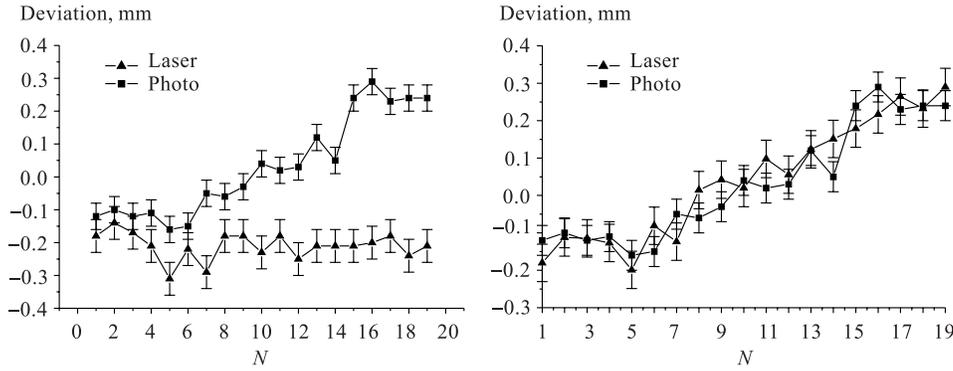
Fig. 11. Line Bel 1 measurement data by the photogrammetric and laser bottom-right methods with no correction applied for MODULE No. 8
