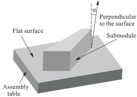
Fig. 3. Definition of submodule maximal twist angle  $\varphi$
