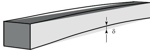
Fig. 7. Sagging («banana») of the girder
