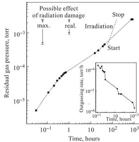
Fig. 5. Residual gas pressure inside the vacuum container as a function of time. The figure inserted shows the outgassing rate behaviour over the same period of time
