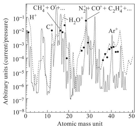
Fig. 3. Composition of the residual gas inside the empty container (filled circles). The dashed line shows results for the residual gas (the spectrometer background) and the dotted line represents the air probe composition measured earlier
