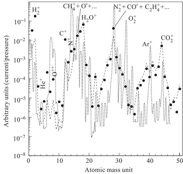
Fig. 4. Gas composition after the annealing procedure (filled circles). The dashed line is the spectrometer background and the dotted line represents the air composition measured earlier
