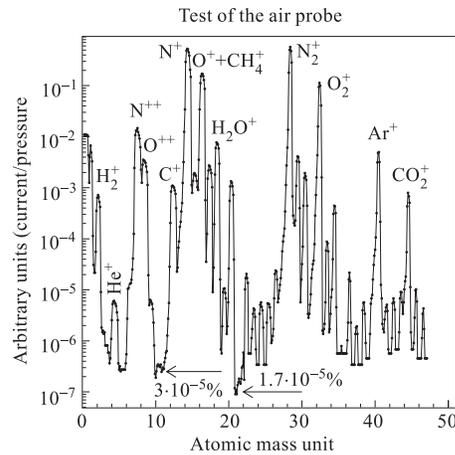
Fig. 2. Composition of the air probe in the operation room. Arrows indicate the mass spectrometer sensitivity level over some specific atomic mass regions
