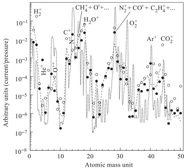
Fig. 6. Residual gas composition measured three months after the irradiation (filled circles). The dashed line is the spectrometer background and the dotted line represents the air probe measured earlier. The measurements carried out before the irradiation (see Fig. 4) are presented (open circles) for comparison
