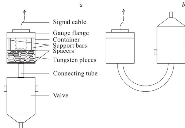
Fig. 1. Schematic drawings of the vacuum container used for *a*) the first and *b*) the second run of irradiation
