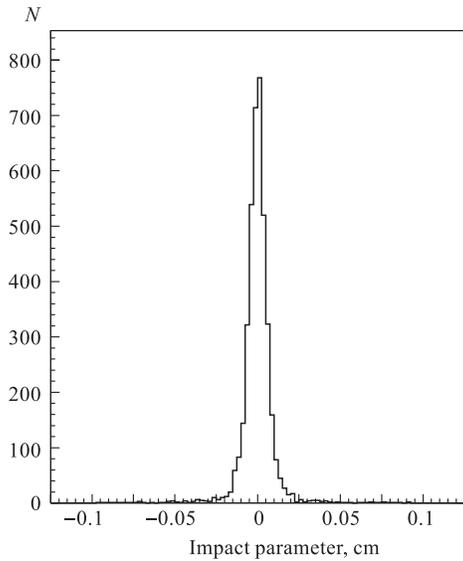
Fig. 6. Impact parameter distribution for data taken in October, 2001, for track candidates with  $\chi^2 < 10$  and  $P_T > 2$  GeV/c, after correction for beam position offset, relative misalignment of the wedges and nonlinearity. In this case the correction for the beam tilt was not necessary since the tilt was  $\simeq 0$ . The Gaussian fit gives  $\sigma = 48 \mu\text{m}$
