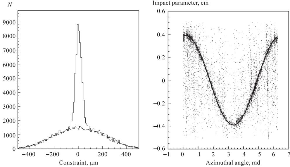
Fig. 1. Constraint distribution in the «silicon-only» configuration. The solid line is for real SVT data, while the dashed line is generated by random hit combinations within the Roads
