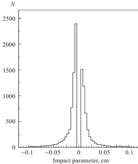
Fig. 9. Impact parameter distribution for tracks which pass the online cuts (number of tracks  $\geq 2$ ,  $\chi^2 < 25$ ,  $P_T > 2 \text{ GeV}/c$ , and  $50 \mu\text{m} < d < 0.1 \text{ cm}$ )
