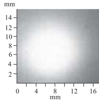
Fig. 3. Television image of the beam spot in the window of the vacuum chamber
