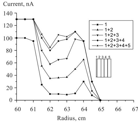
Fig. 2. Measurement of current distribution between probe lamellas
