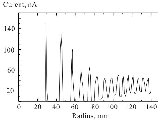
Fig. 1. Current distribution at the centre of the cyclotron after installation of two diaphragms
