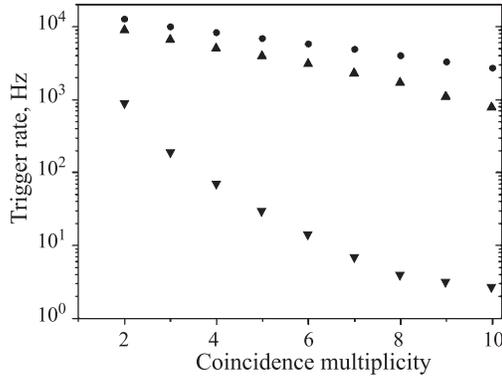
Fig. 2. Dependence of trigger rate on coincidence multiplicity: ● — trigger *c*; ▲ — trigger *u*; ▼ — trigger *d*
