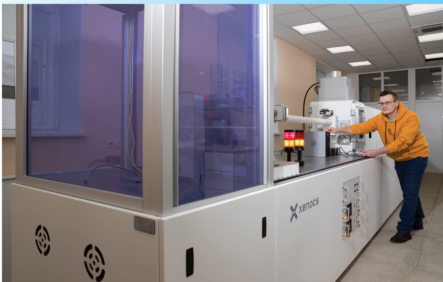
The Xeuss 3.0 X-ray facility, which allows nanoparticles to be studied using X-ray small-angle scattering, as well as to study the crystal structure by X-ray diffraction
