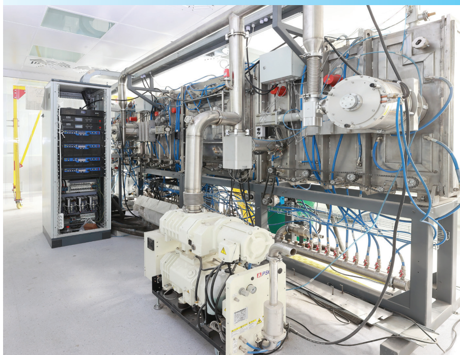
Installation for magnetron sputtering of boron carbide films on substrates made of various materials
