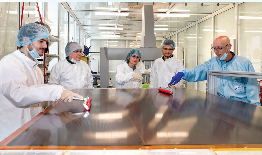
Preparing the reading panel before assembling the MicroMegas detector for the ATLAS experiment
