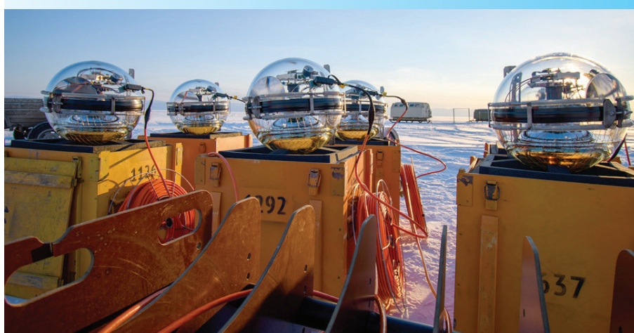
Optical modules prepared for installation of the next Baikal-GVD telescope cluster
