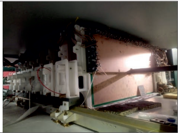
Fig. 2. Left: Vacuum ion beam pipe in front of the BM@N target with built-in silicon strip detectors for measuring the beam trajectory. Right: Tracking detectors based on Gas Electron Multipliers (GEM) installed in the spectrometric magnet using an accurate positioning system
