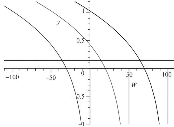
Fig. 1. Solutions of Eq. (41) for different particle spin values. The horizontal straight line is  $y = a_0^{-1/2}$ . The curves are  $y = -2^{-1/2}\zeta[1/2, (1+s)/2 + 1/2a]$  and from left to right  $s = -1, 0, 1$ . The parameter  $W = E'/E_0$  is also shown
