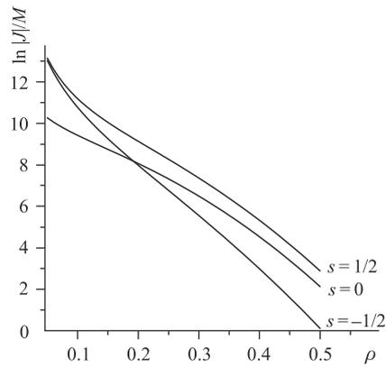
Fig. 10. The dependence of  $\ln(|J|/M)$  on the transverse coordinate obtained using exact formula (24) in the case of the plane  $z = 0$  and the strong field  $h = 100$  for different spin orientations (along the field and opposite the field) and the zero spin
