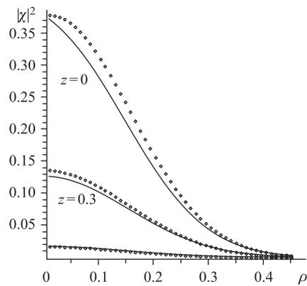
Fig. 7. The dependence of  $|\chi|^2$  on  $\rho$  for the field  $h = 100$  and different  $z$ . The points correspond to the calculation using exact formula (4), and the solid curves correspond to strong field approximations using formulas (10) and (11)
