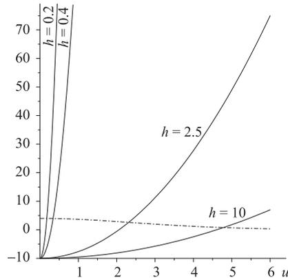
Fig. 3. The solution of transcendental equation (7) in the plane  $z = 1.6$  for  $\rho = 1$ . The solid curves correspond to the left-hand side of Eq. (7) for different values of the magnetic field, and the dash-dotted curve is the graph of the right-hand side of Eq. (7)
