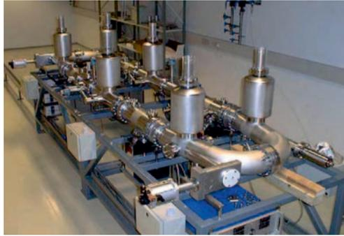
Fig. 1. Photo of compact electrostatic storage ring ELISA kindly presented by S. P. Moller [13]
