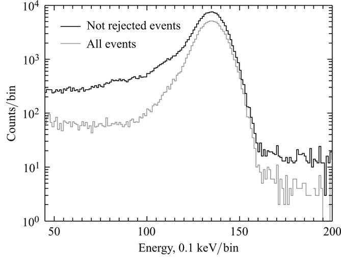
Fig. 5. Original energy spectrum and spectrum after rejection of the events with pulse rise time longer than 47 bins ( $3.8 \mu\text{s}$ ) and  $\lambda$  lower than 115
