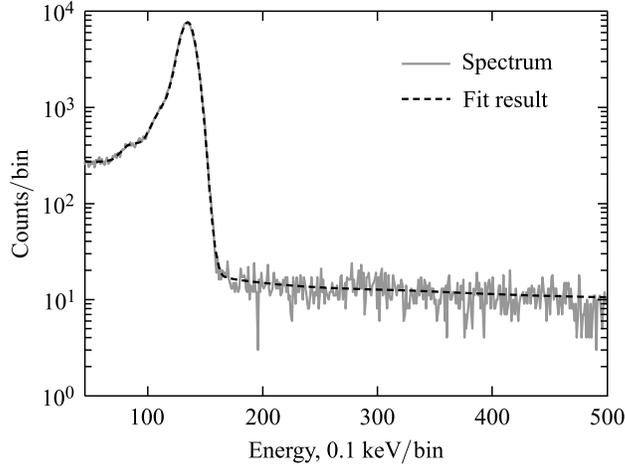
Fig. 2. Background spectra collected with LPC during 26.5 days of measurements and fitting function (13)
