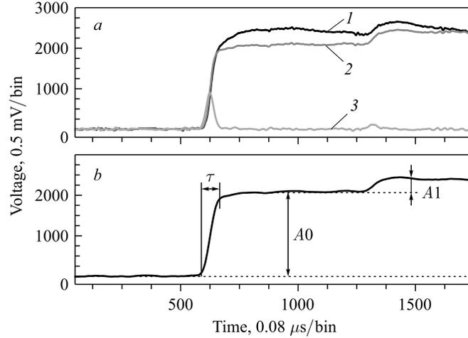
Fig. 1. *a*) Samples of recorded pulse (1), electronic current (3) and corrected pulse (2); *b*) schematic description of the parameters of the corrected pulses used for data analysis.  $A_0$  — amplitude of the primary pulse;  $A_1$  — amplitude of the secondary pulse;  $\tau$  — pulse rise time
