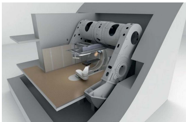
Fig. 19. Gantry-mounted compact proton therapy system. The 9 T synchrocyclotron rotates closely around the patient
