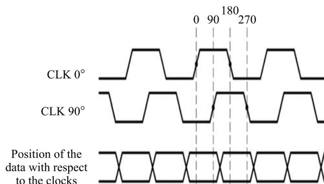
Fig. 10. Oversampling technique using two phase-shifted clocks
