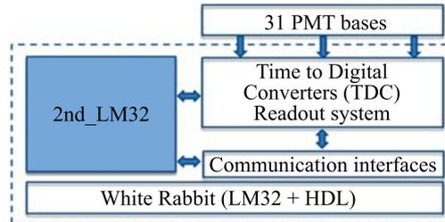
Fig. 9. Block diagram of the CLB firmware
