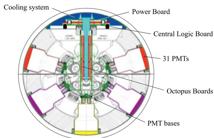
Fig. 2. DOM: position of the Power Board, Central Logic Board, Octopus Board, and PMT bases
