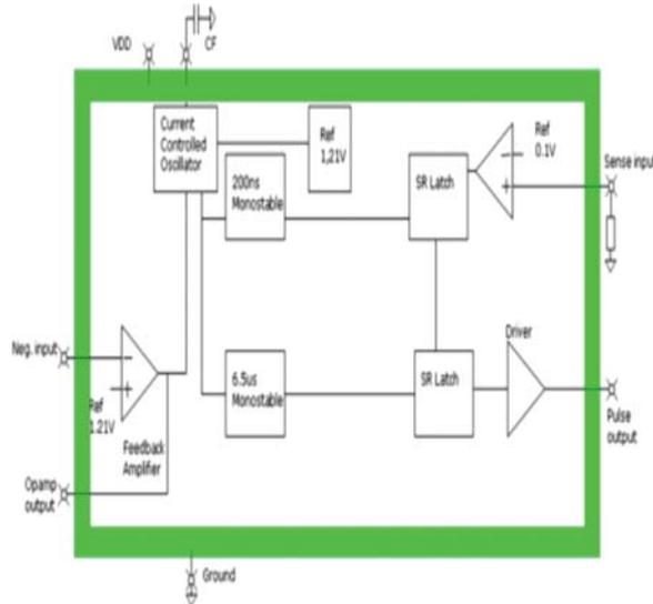
Fig. 5. Block diagram of the CoCo chip
