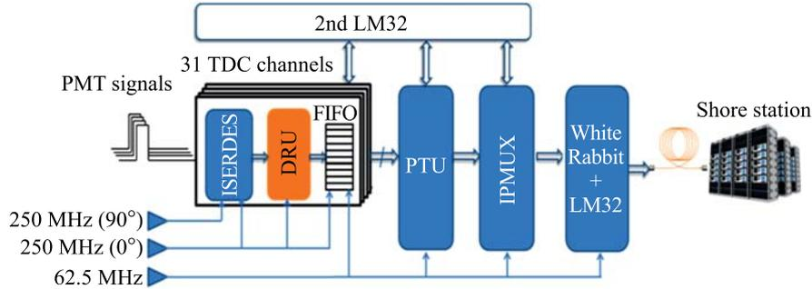
Fig. 11. Complete readout architecture
