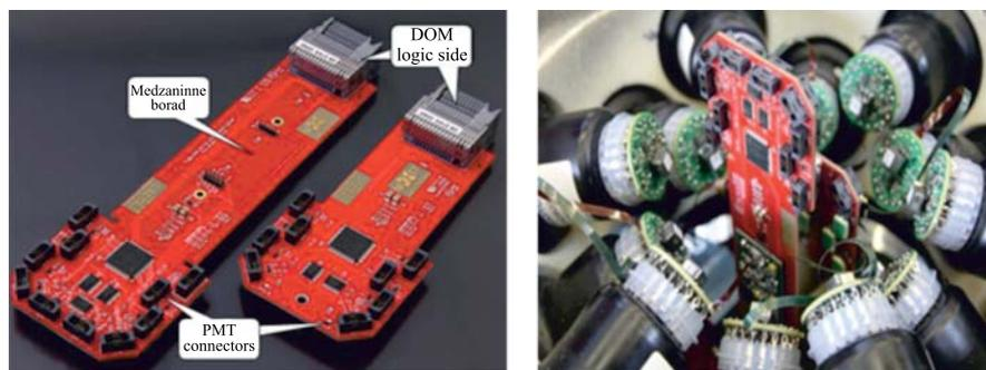
Fig. 6. Large and Short Octopus (left); detail of the Octopus inserted in the DOM (right)
