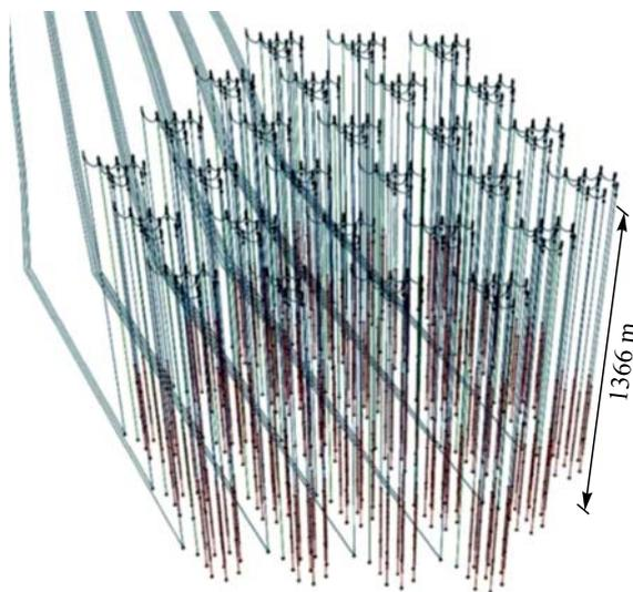
Fig. 1. 3D conceptual model of the GVD telescope (27 clusters)
