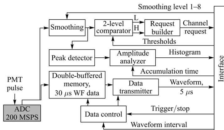
Fig. 3. Functional diagram of one measuring channel of the ADC board
