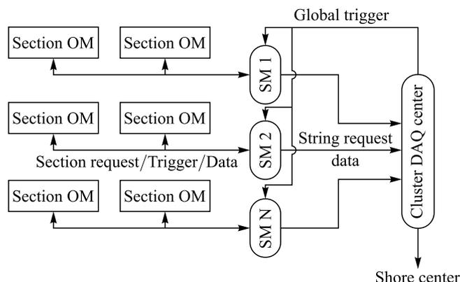
Fig. 4. Diagram of the GVD cluster triggering and data transmission
