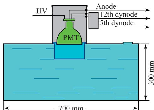
Fig. 3. Standard scintillation counter of the Baksan Underground Scintillation Telescope
