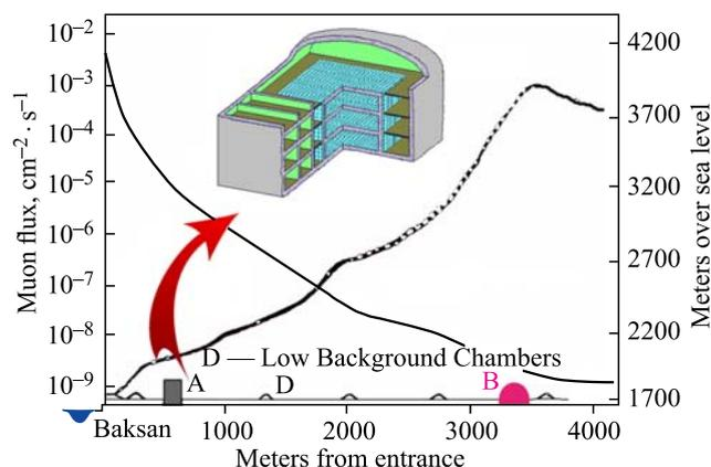
Fig. 1. Schematic illustration of the location of the Baksan Underground Scintillation Telescope
