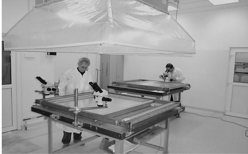
Fig. 2. Wire's plane transfer onto TRD chamber frames
