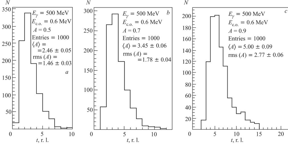
Fig. 1. Distribution of the cascade depth  $t$  at which fixed parts  $A = 0.5$  (a),  $0.7$  (b) and  $0.9$  (c) of the total cascade energy is deposited in liquid xenon when the cascades are produced by gamma quanta of  $E_\gamma = 500$  MeV energy and the cut-off energy is equal to  $E_{c.o.} = 0.6$  MeV. Pointed are also relevant average and rms values. Simulation is performed by using EGS code [3]
