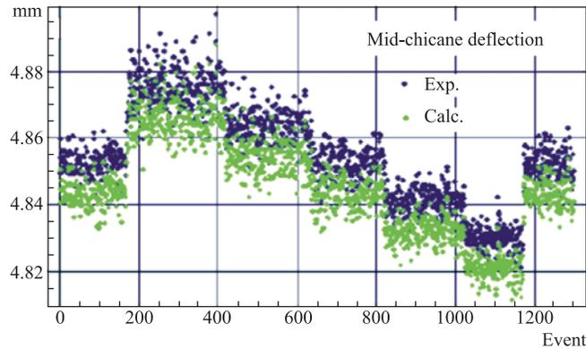
Fig. 8. Measured and calculated mid-chicane beam deflection at energy scan
