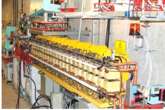
The undulator was designed and constructed by JINR to the FLASH requirements. The undulator period corresponds to  $d = 40 \text{ cm}$ , the number of periods is 9, the magnetic field is varied in the range of 0.1–1.1 T. Output undulator radiation has the following parameters: wavelength 10–200  $\mu\text{m}$ , peak power 1.5 MW, micropulse energy 4  $\mu\text{J}$ , micropulse duration 0.5–6 ps.
