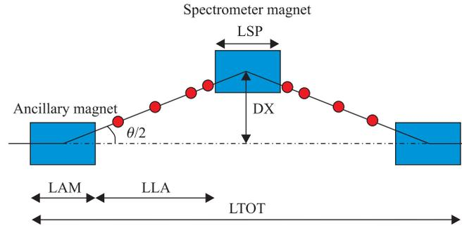
Fig. 7. Scheme of magnetic spectrometer proposed for ILC beam energy measurements
