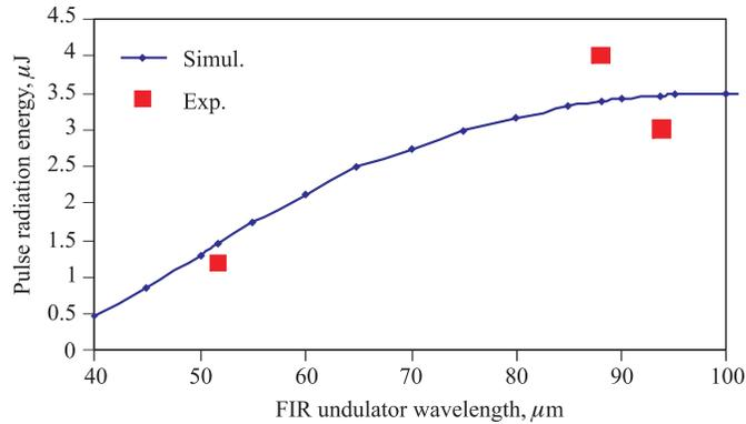
Fig. 5. Dependence of the pulse radiation energy emitted into central cone of the FIR undulator on the wavelength
