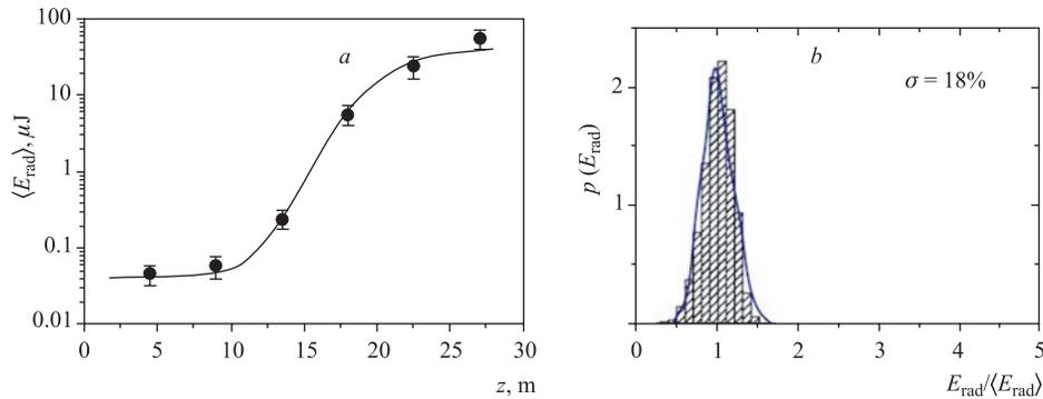
Fig. 2. *a)* Measured average energy in the radiation pulse versus the undulator length showing exponential growth and saturation. *b)* The probability distribution for the energy of the radiation pulses at saturation regime
