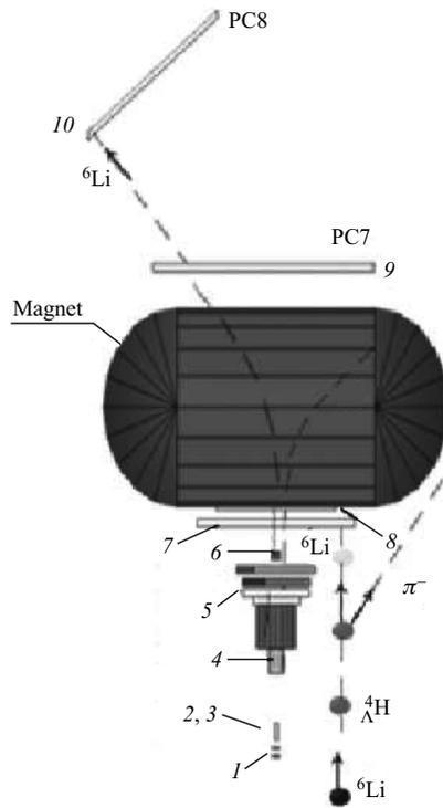
Fig. 1. Layout of HyperNIS spectrometer: 1 — monitors and counters of group A; 2 — target; 3 — counters B; 4 — vacuum vessel; 5 — PC1–PC4; 6 — counters C; 7 — PC5–6; 8 — RPC; 9 — PC7; 10 — PC8
