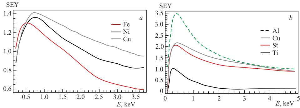
Fig. 1. Color online. *a*) Secondary electron yield vs. primary electron energy for different materials: Fe, Ni, Cu [5]. *b*) Secondary electron yield vs. primary electron energy for perpendicular incidence and for technical surfaces representative for vacuum chambers [2]; materials: titanium (Ti), stainless steel (St), copper (Cu) and aluminum oxide  $\text{Al}_2\text{O}_3$  (Al)
