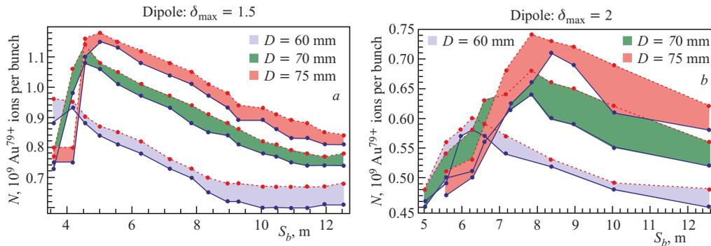
Fig. 2. Color online. Threshold values of  $^{197}\text{Au}^{79+}$  ions per bunch vs. bunch spacing  $S_b$  for  $\delta_{\text{max}} = 1.5$  (*a*) and  $\delta_{\text{max}} = 2$  (*b*)
