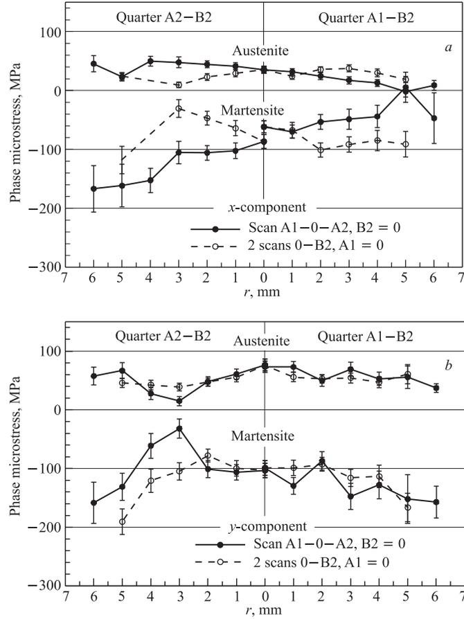
Fig. 5. Dependences of the microstress  $x$ - and  $y$ -components (left and right graphs) in the austenite and martensite phases, respectively, as function of radius  $r$ . Scan along  $y$ -axis was carried out twice for each sample orientation
