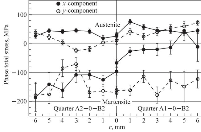
Fig. 2. Radial distributions of  $x$ - and  $y$ -components of the phase total residual stresses in austenite (two upper curves) and martensite (two lower curves) as function of radius  $r$  along A1–0–A2 diameter line with  $y = 0$
