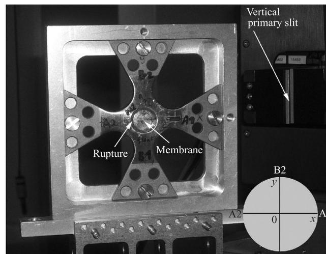
Fig. 1. Photograph showing Kreuz-1 sample mounted on the POLDI instrument for the in-plane *x*-component investigation. In this set-up the A1–A2 sample direction is aligned horizontally along the neutron scattering vector. The vertical slit is visible at the top right with the horizontal slit directly behind it. The *y*-component measurements were done by rotating the sample 90° clockwise to have this direction along the scattering vector
