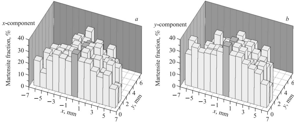
Fig. 3. Two-dimensional distribution of the martensite volume fraction determined using Eq. (6) from respectively the  $x$ - (a) and  $y$ - (b) component investigations within the A1–0–B2 ( $x \geq 0$ ) and A2–0–B2 ( $x \leq 0$ ) membrane quarters
