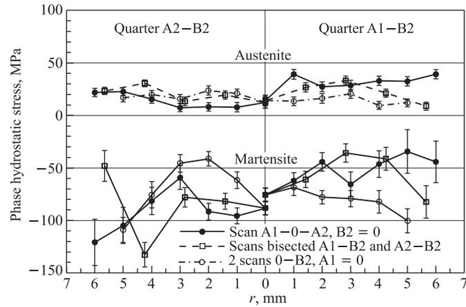
Fig. 6. Radial distributions of the hydrostatic stresses in the austenite and martensite phases along the respective load directions, as well as along a measurement direction bisecting the primary load directions
