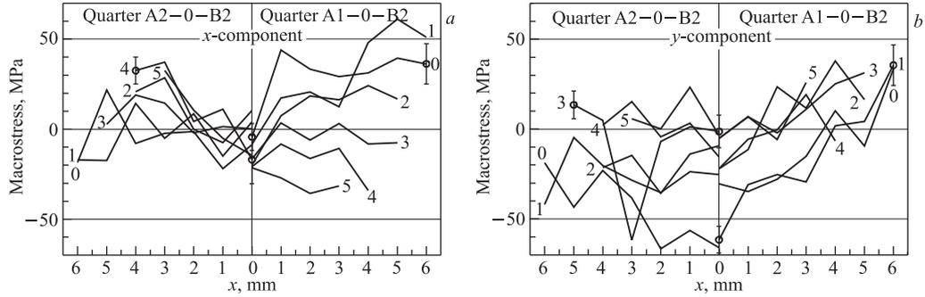
Fig. 4. Dependences of the  $x$ - and  $y$ -component macrostresses (plots  $a$  and  $b$ , respectively) on  $x$ -coordinate in the top half section of the membrane at different  $y$ -coordinates shown as a number of a curve. Typical error is shown for some curves
