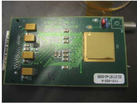
Fig. 9. Spectrometric detector on the basis of GaAs(Cr) pixel sensor with  $256 \times 256$  channels of  $50 \mu\text{m}$  resolution and Medipix chip
