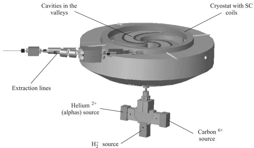
Fig. 1. Artist's view of the median plane in the carbon/proton superconducting cyclotron
