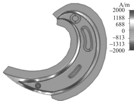
Fig. 10. Magnetic field in the median plane
