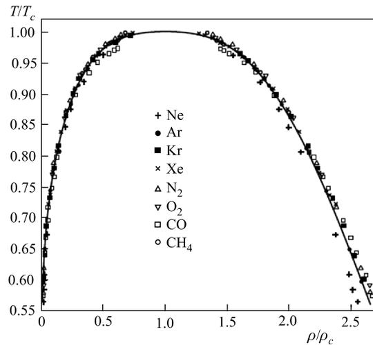
Fig. 1. The coexistence curve (the scaled density  $\rho/\rho_c$  vs. the scaled temperature  $T/T_c$ ) for different fluids [30]. The solid curve is fitted with the cubic equation  $\rho/\rho_c \sim |T/T_c|^{1/3}$
