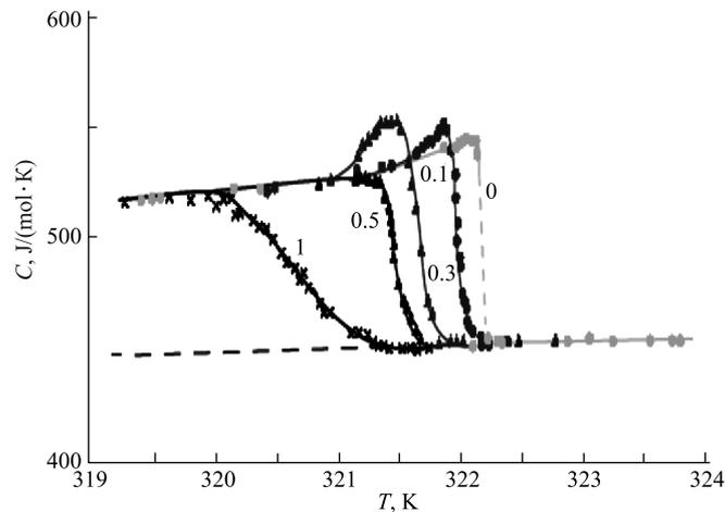
Fig. 4. Specific heat of ferroelectric crystal  $(\text{CH}_2\text{NH}_2\text{COOH})_3\text{H}_2\text{SO}_4$  undergoing radiation as a function of the temperature [34]. The dose of irradiation is shown in megaröntgens
