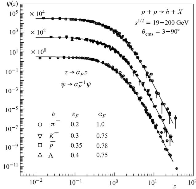
Fig. 5. Inclusive spectra of the hadrons produced in proton–proton collisions in the  $z$ -presentation. The symbols denote the experimental data obtained in the experiments performed at CERN, FNAL, and BNL [6, 7]
