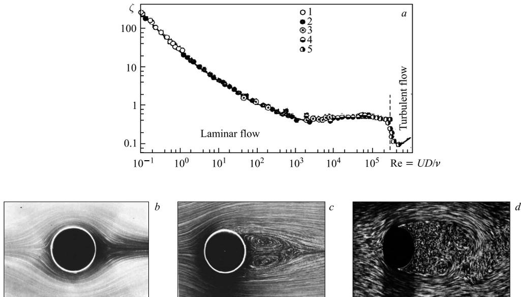
Fig. 2. *a*) Variation of the drag coefficient  $\zeta$  with Reynolds number  $Re$  for sphere [32]. Points are the experimental data. The uniform flow passes over the circular cylinder at  $Re = 0.16$  (*b*),  $Re = 26$  (*c*), and  $Re = 2000$  (*d*) [33]
