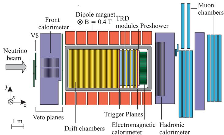
Fig. 2. Side view of the NOMAD detector
