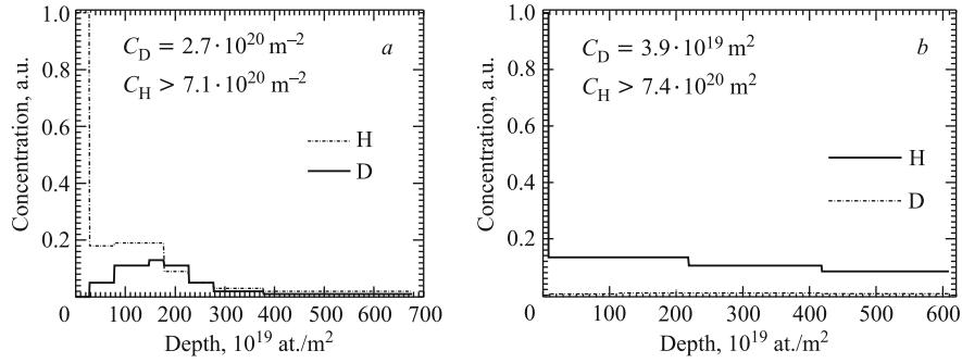
Fig. 9. ERDA depth concentrations of D and H atoms after implantation of D<sup>+</sup> ions up to a fluence of  $\Phi = 1.2 \cdot 10^{22} \text{ m}^{-2}$  (*a*) and saturation under 9 kbar deuterium gas during three days of Pd<sub>0.9</sub>Ru<sub>0.1</sub> sample (*b*). Measurements were carried out 30 days after saturation and implantation
