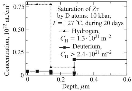
Fig. 8. ERDA depth concentrations of D and H atoms after saturation of annealed (at 125°C, one hour) pure zirconium sample under 10 kbar deuterium gas high pressure during twenty days at temperature 127°C. Measurements were carried out 5 days after saturation
