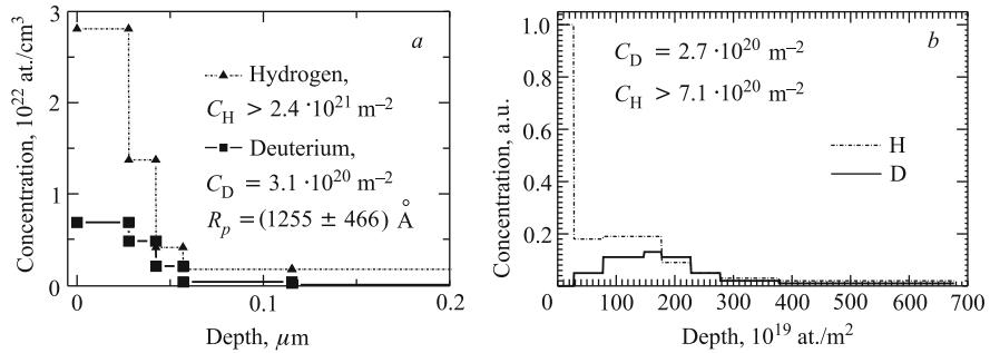
Fig. 15. The depth concentrations of D and H atoms after  $D^+$ -ion implantation with the energy of 25 keV at a fluence of  $\Phi_1 = 1.2 \cdot 10^{22} \text{ m}^{-2}$  in Pd<sub>0.9</sub>Ru<sub>0.1</sub> samples 10 days after (a) and three month later (b)
