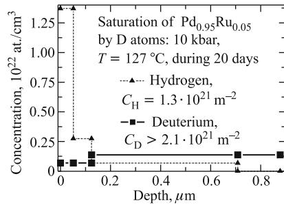
Fig. 7. ERDA depth concentrations of D and H atoms after saturation of annealed (at 125°C, one hour) Pd<sub>0.95</sub>Ru<sub>0.05</sub> sample under 10 kbar deuterium gas high pressure during twenty days at temperature 127°C. Measurements were carried out 5 days after saturation
