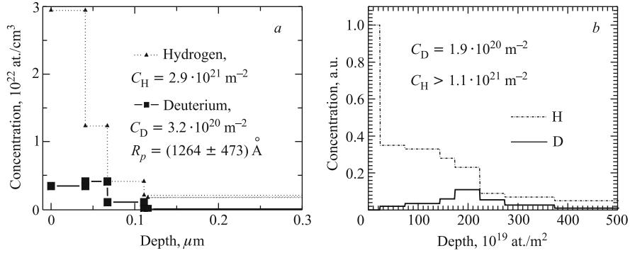
Fig. 14. The depth concentrations of D and H atoms after  $D^+$ -ion implantation with the energy of 25 keV at a fluence of  $\Phi_1 = 1.2 \cdot 10^{22} \text{ m}^{-2}$  in Pd<sub>0.9</sub>Rh<sub>0.1</sub> samples 10 days after (a) and three month later (b)
