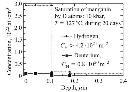
Fig. 6. ERDA depth concentrations of D and H atoms after saturation of annealed (at 125°C, one hour) manganin sample under 10 kbar deuterium gas high pressure during twenty days at 127°C temperature. Measurements were carried out 5 days after saturation
