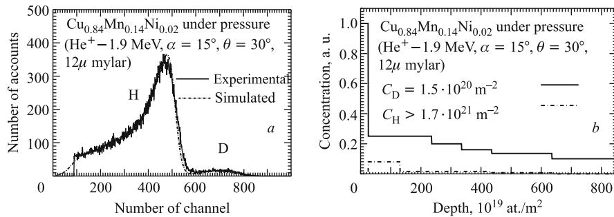
Fig. 3. The experimental and simulated spectra of H and D recoils measured by ERDA (*a*) and calculated depth concentrations of D and H atoms after saturation of manganin alloy sample under 9 kbar deuterium gas high pressure during 72 h (*b*). Measurements were carried out a long period of time after saturation
