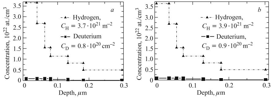
Fig. 4. ERDA depth concentrations of D and H atoms after saturation of annealed manganin sample (at  $125^\circ\text{C}$ , one hour) under 9 kbar deuterium gas high pressure during 72 h. Measurements were carried out one month after saturation on the same sample just in different places ((a) and (b)) for detailed comparison of result repetition
