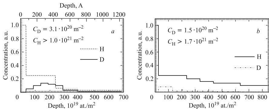
Fig. 10. ERDA depth concentrations of D and H atoms after implantation of D<sup>+</sup> ions up to a fluence of  $\Phi = 1.2 \cdot 10^{22} \text{ m}^{-2}$  (*a*) and saturation under 9 kbar deuterium gas during three days of Pd<sub>0.9</sub>Ag<sub>0.1</sub> sample (*b*). Measurements were carried out three months after implantation and saturation
