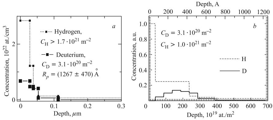
Fig. 13. The depth concentrations of D and H atoms after  $D^+$ -ion implantation with the energy of 25 keV at a fluence of  $\Phi_1 = 1.2 \cdot 10^{22} \text{ m}^{-2}$  in Pd<sub>0.9</sub>Pt<sub>0.1</sub> samples 10 days after (a) and three months later (b)
