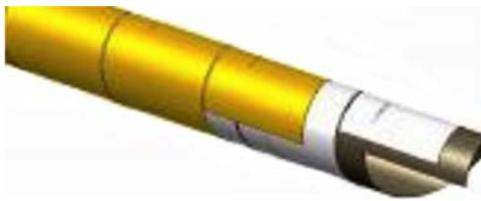
Fig. 5. Straw tube consisting of a carbon-loaded inner layer 40  $\mu\text{m}$  thick and an aluminized Kapton outer layer  $\sim 25 \mu\text{m}$  thick
