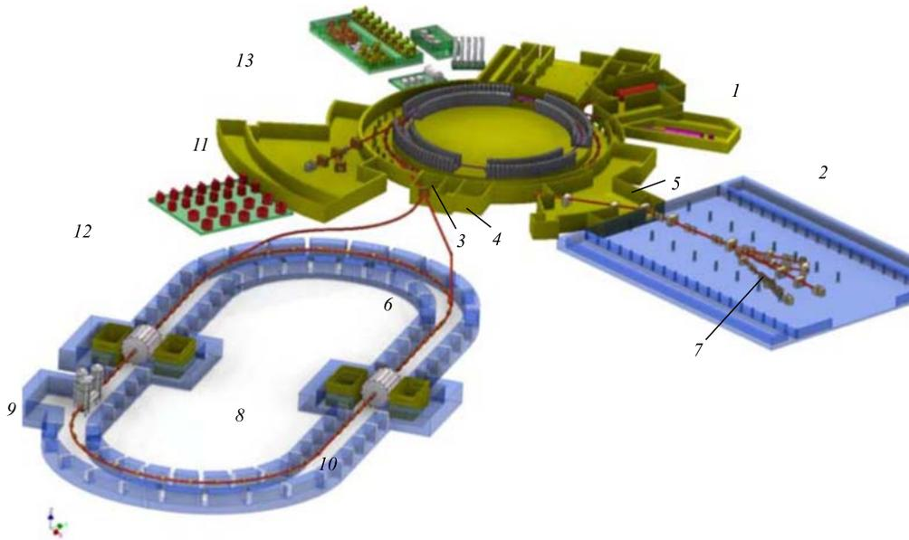
Fig. 1. Scheme of the NICA facility: 1 — light and polarized ion sources and «old» Alvarez-type linac; 2 — ESIS source and new RFQ linac; 3 — Synchrofasotron yoke; 4 — booster; 5 — Nuclotron; 6 — beam transfer lines; 7 — Nuclotron beam lines and fixed target experiments; 8 — collider; 9 — MPD; 10 — SPD; 11 — new research area; 12 — cryogenic plant; 13 — auxiliary equipment
