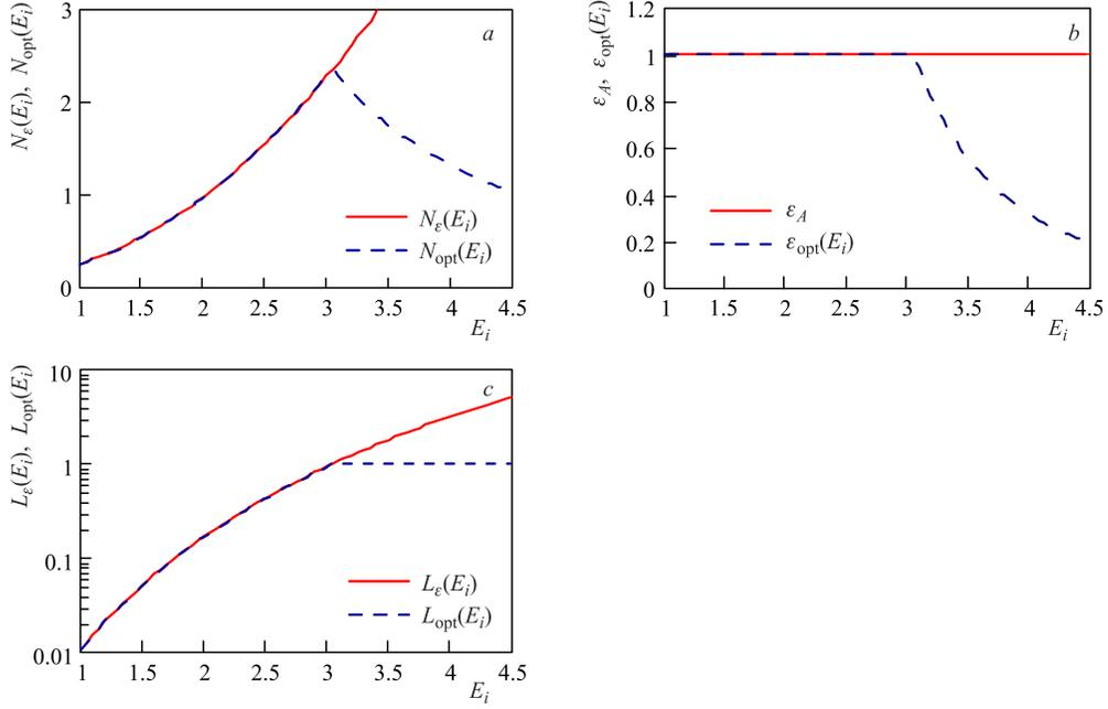
Fig. 2. Space charge dominated regime; ion number per bunch (a), emittance (b) and luminosity (c) versus ion energy in two cases: full acceptance if filled with ions (red solid curve) and luminosity is limited (blue dashed curve); the ring acceptance =  $40 \pi \cdot \text{mm} \cdot \text{mrad}$ , parameter units:  $[N_i] = 10^9$ ,  $[\epsilon] = \pi \cdot \text{mm} \cdot \text{mrad}$ ,  $[L] = 10^{27} \text{ cm}^{-2} \cdot \text{s}^{-1}$
