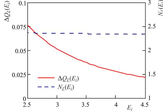
Fig. 3. IBS dominated regime; beam tune shift  $\Delta Q_{tot}$  (red solid curve) and ion number per bunch  $N_i$  (blue dashed curve) at constant luminosity  $L = 1 \cdot 10^{27} \text{ cm}^{-2} \cdot \text{s}^{-1}$  and beam emittance of  $1.0 \pi \cdot \text{mm} \cdot \text{mrad}$ ;  $[N_i] = 10^9$
