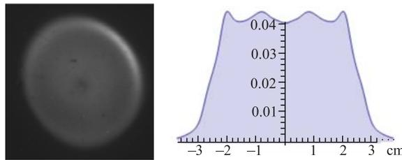
Fig. 4. The light output from the scintillator and the density distribution of the ion  $C^{+6}$  at 8.5  $\mu$ s after beginning of discharge at a distance of 110 cm for a current of 80 kA. The spot rms diameter is 40 mm
