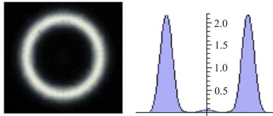
Fig. 8. The light output from a scintillator and the distribution of ion  $\text{Fe}^{+26}$  density calculated in the model approximation for the experimental condition
