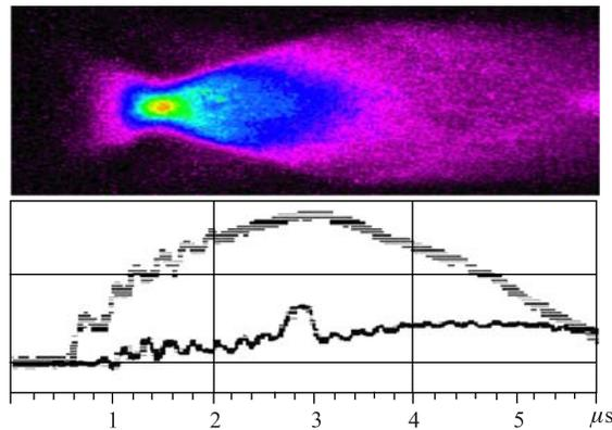
Fig. 2. Time scanning of a discharge luminescence and a discharge and beam currents for short pulse mode
