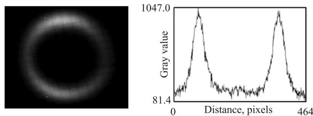
Fig. 6. Light output from scintillator and the density distribution of ion  $Fe^{+26}$  at  $1.7 \mu s$  after beginning of discharge at a distance of 30 cm for a current of 150 kA. The ring diameter is 9 mm
