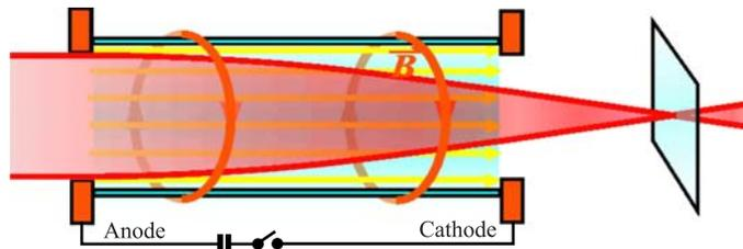
Fig. 1. Ion focusing in a plasma lens
