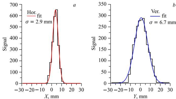
Fig. 4. The  $X$ - (a) and  $Y$ - (b) coordinate beam profile at the focus F5. The lines are the same as in Fig. 3
