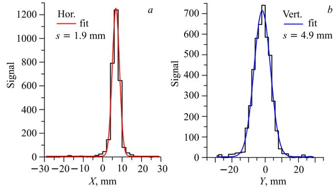
Fig. 3. The  $X$ - (a) and  $Y$ - (b) coordinate beam profile at the focus F4. The lines are the results of the Gaussian fit
