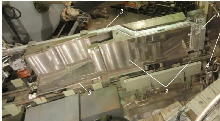
Fig. 5. Moveable trolley with cold moderator and the biological shielding installed on the rails in ready-to-move-to-active-core position: 1 — cold moderator with vacuum shielding and water premoderator; 2 — cold helium and beads support pipelines; 3 — trolley on the rails; 4 — entrance of a passing through the stationary biological shielding of reactor to the active core; 5 — drain pipeline of liquid mesitylene
