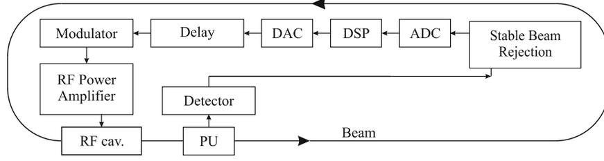
Fig. 2. Longitudinal feedback system layout
