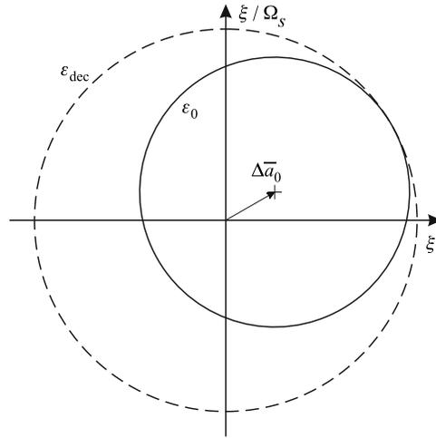
Fig. 1. Injected emittance  $\varepsilon_0$  dilution to  $\varepsilon_{dec}$  because of error  $\Delta\bar{a}_0$
