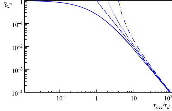
Fig. 5. Dependence of  $F_\varepsilon^2$  on  $\tau_{\text{dec}}/\tau_d$  without instability (solid curve),  $\tau_{\text{inst}} = \tau_{\text{dec}}$  (dashed),  $\tau_{\text{inst}} = \tau_{\text{dec}}/2$  (dotted),  $\tau_{\text{inst}} = \tau_{\text{dec}}/4$  (dash-dotted)
