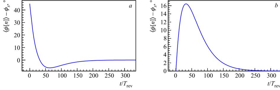
Fig. 6. Signals from pick-up (critical damped mode): phase (a) and energy (b) errors
