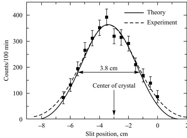
Fig. 3. Measured and predicted intensity distribution as a function of the crystal outlet surface slit position
