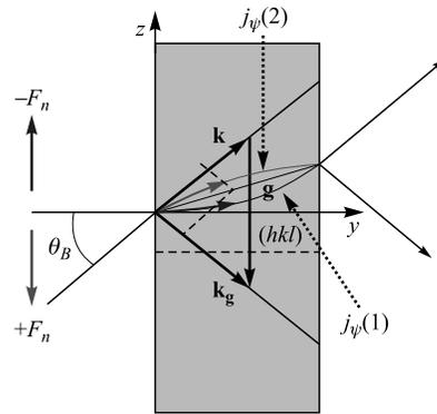
Fig. 1. Scheme of Laue diffraction in a single crystal in the presence of external force acting along the reciprocal lattice vector.  $j_{\psi(1)}$  and  $j_{\psi(2)}$  are the so-called «Kato trajectories» for the different types of Bloch waves
