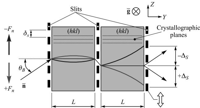
Fig. 2. Two-crystal scheme of Laue diffraction. Collimating slits are situated at the inlet and outlet crystal faces
