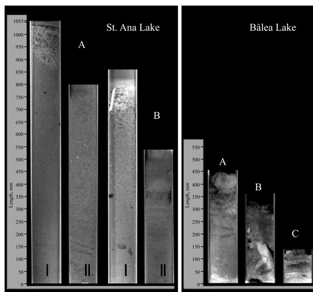
Fig. 2. Digital radiographs of investigated cores. Due to their length, St. Ana Lake cores (left) were sectioned into two fragments (I and II), while Bâlea Lake cores (right), significantly shorter, were investigated uncut
