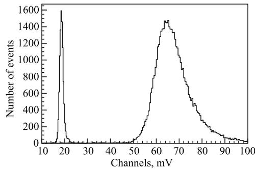
Fig. 16. Spectrum of LYSO and GSO crystals on the  $^{137}\text{Cs}$  source at constant parameters of the measuring system
