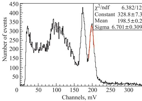
Fig. 2. Energy spectrum of LYSO crystal on  $^{60}\text{Co}$  source
