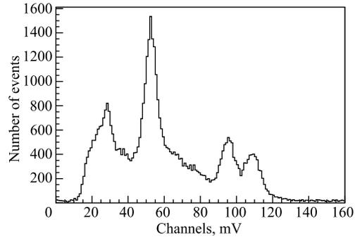
Fig. 11. Energy spectrum of LYSO crystal on the  $^{133}\text{Ba}$ ,  $^{137}\text{Cs}$ ,  $^{60}\text{Co}$  sources
