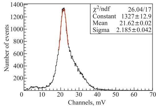
Fig. 7. Signal spectrum of GSO crystal on  $^{137}\text{Cs}$  source with a collimator with an aperture of 2 mm
