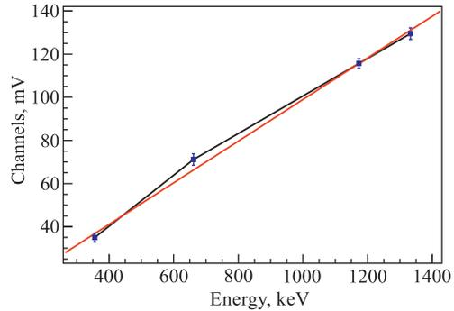
Fig. 13. Energy calibration of LYSO crystal on the  $^{133}\text{Ba}$ ,  $^{137}\text{Cs}$ ,  $^{60}\text{Co}$  sources
