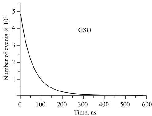
Fig. 21. Arrival time spectrum of photons for calorimeter on GSO crystals
