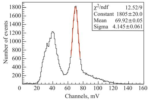
Fig. 3. Energy spectrum of LYSO crystal on  $^{137}\text{Cs}$  and  $^{133}\text{Ba}$  sources
