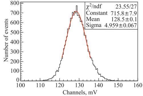
Fig. 5. Energy spectrum of LYSO crystal on a collimated  $^{22}\text{Na}$  source
