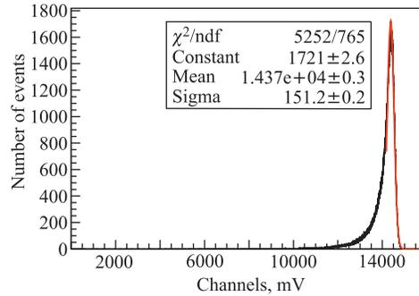
Fig. 20. Simulated optical spectrum on the 105-MeV electron source for the COMET calorimeter on LYSO crystals
