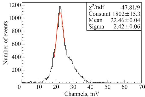
Fig. 6. Signal spectrum of GSO crystal on  $^{137}\text{Cs}$  source without a collimator
