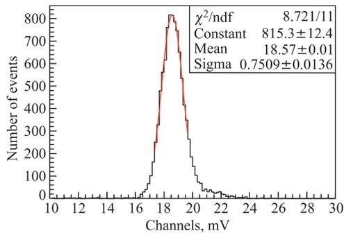
Fig. 8. Spectrum of signal of GSO crystal on the  $^{137}\text{Cs}$  source with a collimator with an aperture of 0.5 mm
