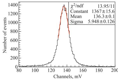
Fig. 9. Spectrum of signal of GSO crystal on the  $^{22}\text{Na}$  source with a collimator with an aperture of 1 mm
