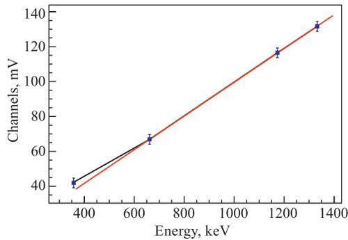
Fig. 12. Energy calibration of GSO crystal on the  $^{133}\text{Ba}$ ,  $^{137}\text{Cs}$ ,  $^{60}\text{Co}$  sources
