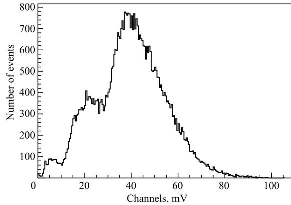
Fig. 1. Spectrum of LYSO crystal intrinsic radioactivity
