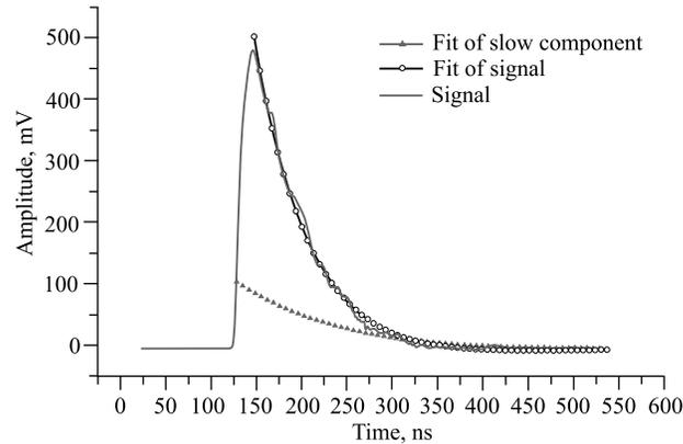
Fig. 17. Timing signal of GSO crystal on the  $^{137}\text{Cs}$  source with constant parameters of the measuring system
