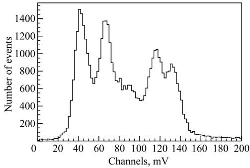
Fig. 10. Energy spectrum of GSO crystal on the  $^{133}\text{Ba}$ ,  $^{137}\text{Cs}$ ,  $^{60}\text{Co}$  sources
