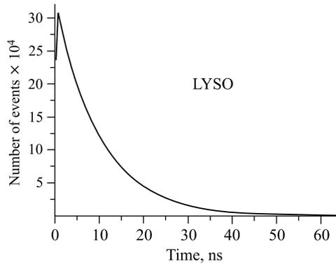
Fig. 22. Arrival time spectrum of photons for calorimeter on LYSO crystals
