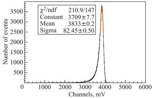
Fig. 19. Simulated optical spectrum on the 105-MeV electron source for the COMET calorimeter on GSO crystals
