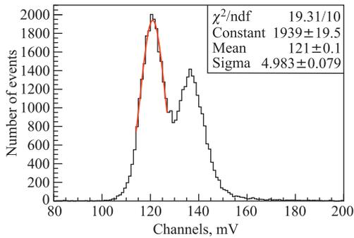
Fig. 4. Energy spectrum of LYSO crystal on a collimated  $^{60}\text{Co}$  source
