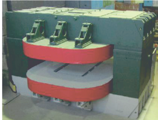
Fig. 5. The view of modernized SP41 dipole magnet
