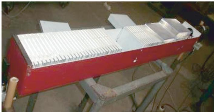
Fig. 8. Inside view of the calorimeter module prototype
